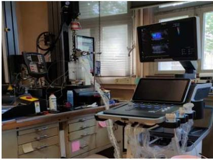
Figure 2: Mechanical testing device (Instron 5944) coupled with an ultrafast ultrasound device (Mach 30) driving a 6 MHz central frequency US linear probe.
