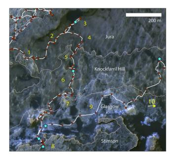
**Figure 5.** Curiosity's traverse area within Glen Torridon. The white line is the rover traverse path and the red circles are stops along the traverse. The numbers correspond to the 10 waypoints defined in Section 4.1 (HiRISE image ESP\_060840\_1750). Stars indicate drill sample locations. The stratigraphic members are labeled, and the member boundaries are denoted by the pink lines.
