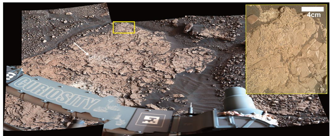
Figure 21. Mastcam mosaic (2865ML14954, NASA/JPL-Caltech/MSSS) of the Mary Anning 3 drill site (white arrow). The drill hole is \sim 1.6 cm in diameter. The yellow box indicates where MnO-rich nodules were identified by the ChemCam instrument and later drilled; Inset shows Mars Hand Lens Imager image 2906MH0004240011003483C00 of the Groken drill target before the sample was collected. Nodules are visible as the dark spots on the rock.
