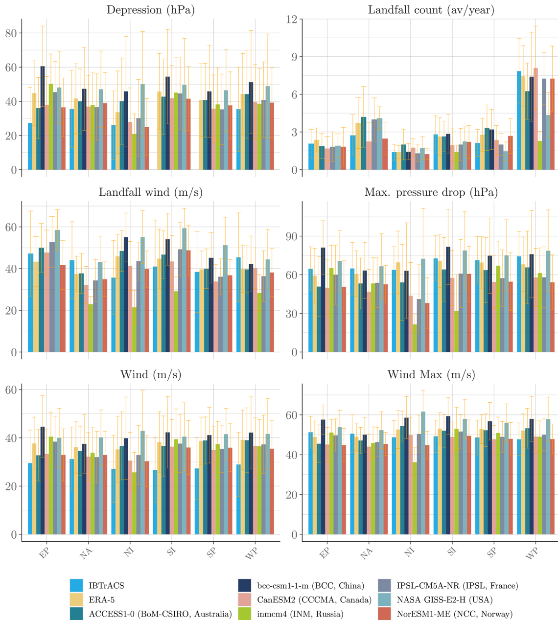
Figure A6. Evidence of model uncertainty. A comparison of the properties obtained by generating 30 years of tropical cyclones with different models from the CMIP5 raw climate data vs. ERA5. The average number of cyclones making landfall is computed by averaging the number of events with a number of steps on land positive ( s_1 > 0 ). Maximum pressure drop and wind are, respectively, computed by extracting the maximum value for the corresponding variables of the cyclone tracks. The light blue bars represent the mean of the variable of interest among the IBTrACS-filtered dataset (with the confidence interval drawn from the standard deviation of the distribution). The yellow bars represent the same variable extracted from the synthetic data generated by Algorithm 1 using ERA5 data. In terms of average values, the models produce consistent tracks in every basin. Then, we compare the output of this algorithm with different climate data produced on the historical period by the climate models taking part in the fifth phase of the CMIP. A general observation is the poorer performance of the model in the northern Indian basin. This could be due to the smaller number of intense cyclones remaining in the sample after the filtration by intensity (1.6 storms per year with winds exceeding 35 \text{ ms}^{-1} ).
