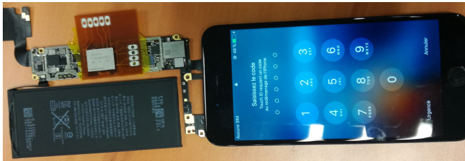
Fig. 4. iPhone 6s with a test interposer between the motherboard and its memory.
