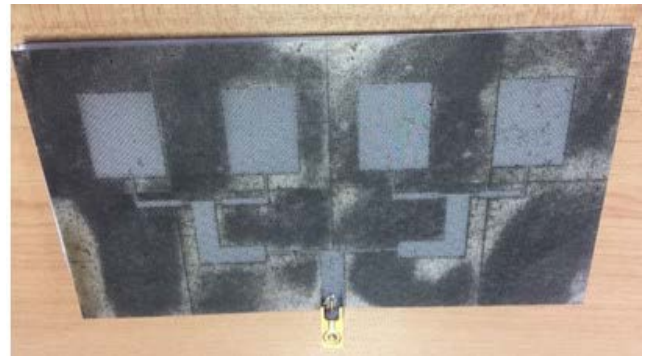
FIGURE 9. Photograph of the FPMC antenna array. The laser-etched areas are in dark color and the pristine areas which define the antenna array pattern are in a bright color.
