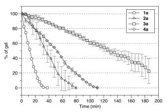
Figure 7 Percentage of remaining gel against time (min) after immersion in water. Gels prepared with 1a-4a at 12 mg mL<sup>-1</sup> in toluene.
