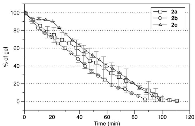
**Figure 8** Percentage of remaining gel against time (min) after immersion in water. Gels prepared with **2a, 2b, 2c** at 16 mg mL<sup>-1</sup> in toluene.
