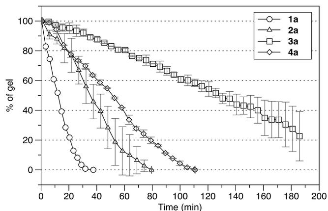
**Figure 7** Percentage of remaining gel against time (min) after immersion in water. Gels prepared with **1a-4a** at 12 mg mL<sup>-1</sup> in toluene.
