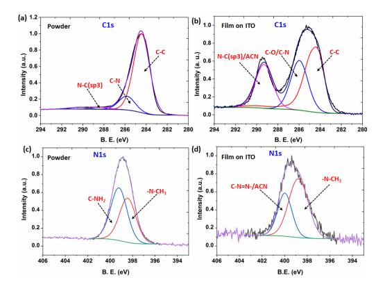
**Figure 3:** C1s spectra (a and b) and N1s spectra (c and d), and their deconvolution into different components for m-Cz diamine powder and m-Cz film electrografted on ITO substrate.
