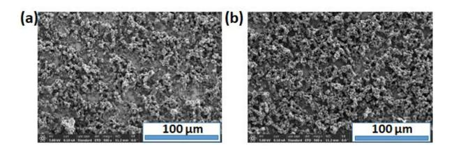
**Figure 9:** SEM images of the polyCz films electrodeposited on bare ITO (a) and m-Cz-ITO (b) surfaces.
