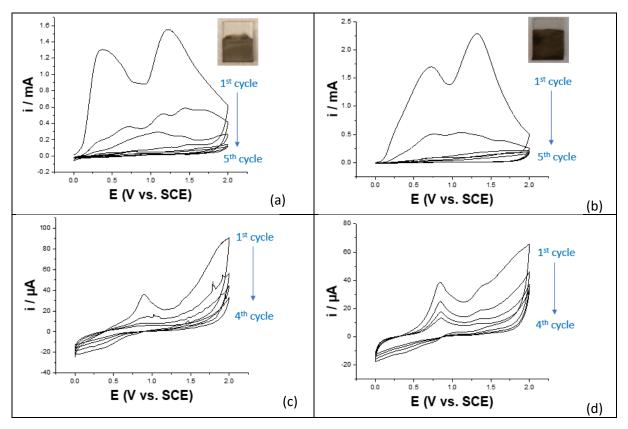
**Figure 5:** Electrochemical oxidation of 9-methyl-9*H*-carbazole-3,6-diamine (0.01 M) in acetonitrile + 0.1 M LiClO<sub>4</sub>: (a) on bare ITO, (b) on m-Cz-ITO. Post-polymerization cyclic voltammetry of the resulting films in acetonitrile + 0.1 M LiClO<sub>4</sub>: (c) on bare ITO, (d) on m-Cz-ITO.
