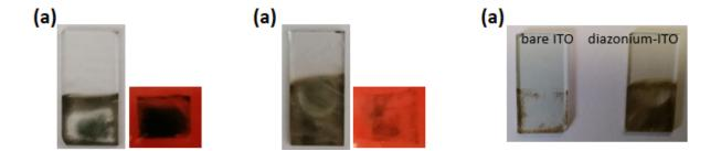
**Figure 10:** Adhesion test with a scotch tape of a polyCz film electrodeposited on bare ITO (a) and m-Cz-ITO (b). Picture of the same films after immersion in water for 2 months (c).
