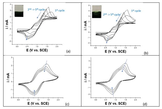
**Figure 8:** Electrochemical oxidation of carbazole monomers (0.01 M) in acetonitrile + 0.1 M LiClO<sub>4</sub>: (a) on bare ITO, (b) on m-Cz-ITO. Post-polymerization cyclic voltammetry of the resulting films in acetonitrile + 0.1 M LiClO<sub>4</sub>: (c) on bare ITO, (d) on m-Cz-ITO.
