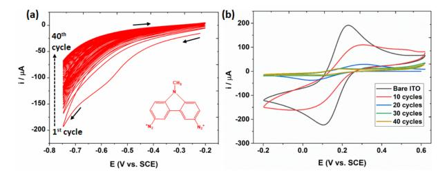
**Figure 1**: Voltammograms (40 cycles) of ITO-coated glass electrode recorded in 0.1 M LiClO<sub>4</sub> in ACN + 2 mM 9-methyl-9*H*-carbazole diazonium in a potential window of -0.2 V to -0.75 V at a scan rate of 40 mV s<sup>-1</sup> (a). Comparison of CVs of 9-methyl-9*H*-carbazole grafted on ITO electrodes at different cycles and bare ITO electrode in 0.1 M KCl + 5 mM K<sub>3</sub>[Fe(CN)<sub>6</sub>] at scan rate of 40 mV s<sup>-1</sup>(b).
