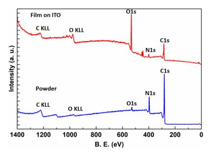
**Figure 2:** Comparison of XPS survey spectra of m-Cz film electrografted on ITO and m-Cz diamine powder.
