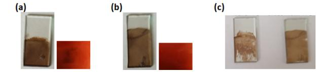
**Figure 7:** Adhesion test with a scotch tape of a poly(m-Cz diamine)film electrodeposited on bare ITO (a) and m-Cz-ITO (b). (c): Left: picture of the film (a) after immersion in water for 2 months, right: picture of the film (b) after immersion in water for 2 months.
