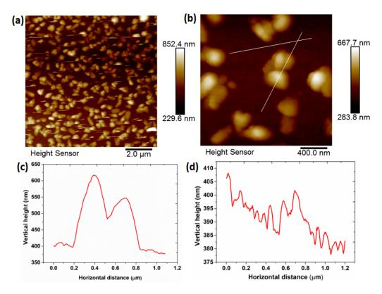
Figure 4: AFM images (a and b) and surface height variations (c and d) of m-Cz-ITO surface.
