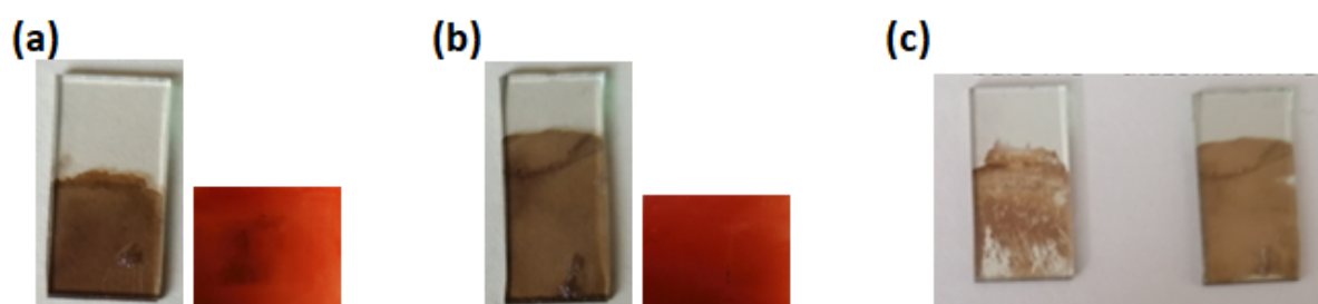
Figure 7: Adhesion test with a scotch tape of a poly(m-Cz diamine)film electrodeposited on bare ITO (a) and m-Cz-ITO (b). (c): Left: picture of the film (a) after immersion in water for 2 months, right: picture of the film (b) after immersion in water for 2 months.
