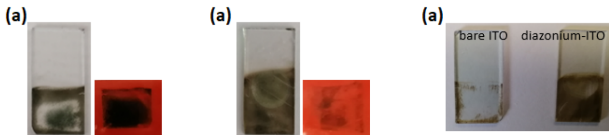
Figure 10: Adhesion test with a scotch tape of a polyCz film electrodeposited on bare ITO (a) and m-Cz-ITO (b). Picture of the same films after immersion in water for 2 months (c).
