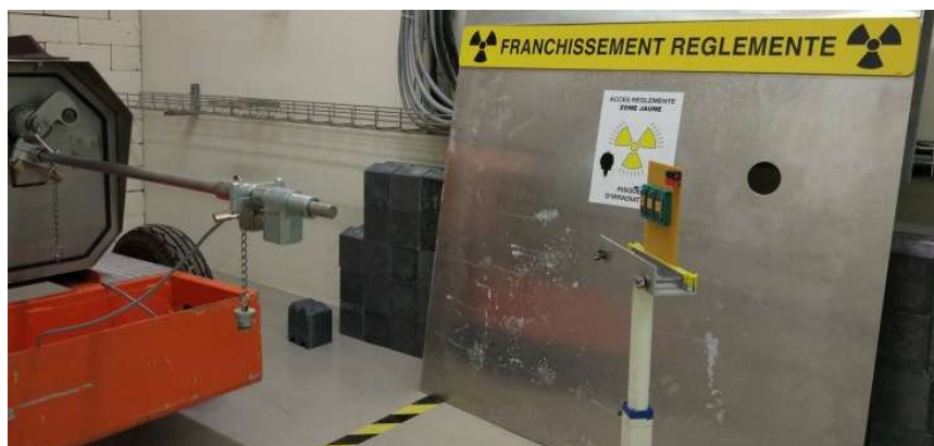
Figure 3 : MEGA facility for Total Ionizing Dose tests and analysis at ONERA in Toulouse, France.
