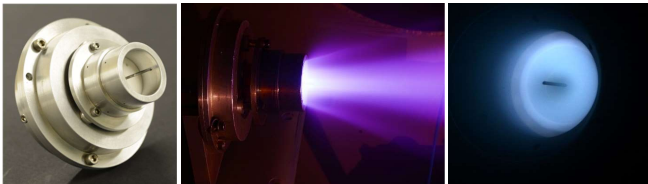
Figure 7 : Left, the microwave electrical thruster, ECRA. Middle, the 30 W version. Right, the 200 W version
