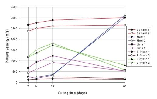
Figure 6. P-wave velocity as a function of curing time for individual binders.
