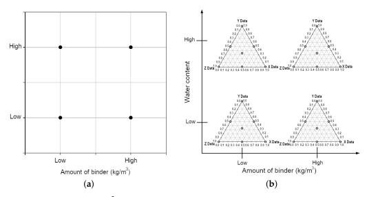
**Figure 5.** An example of a  $2^2$ -factor experiment with binder quantity and water ratio as factors (a); An example of a  $2^2$ -factor trial in combination with simplex trials (b).
