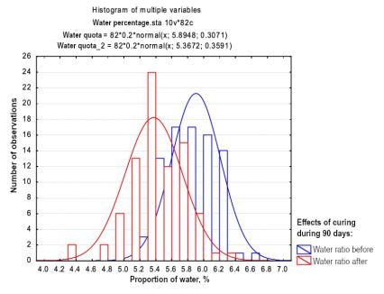
**Figure 3.** Histogram of water content in soil specimens.
