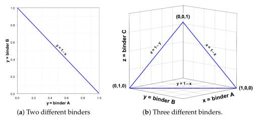
Figure 4. Application of simplex lattice design showing possible binder combinations.
