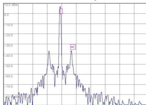
Figure 5: Spectral analysis of the master oscillator driver, with 1 Hz resolution and video bandwidths.
