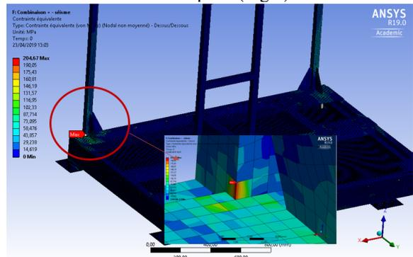
Figure 7: Max stress in the supporting beam.
