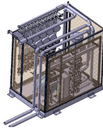
Figure 6: Exchanger structure and retention tray.
