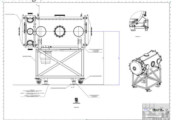
Figure 3: FALSTAFF detection assembly drawing.
