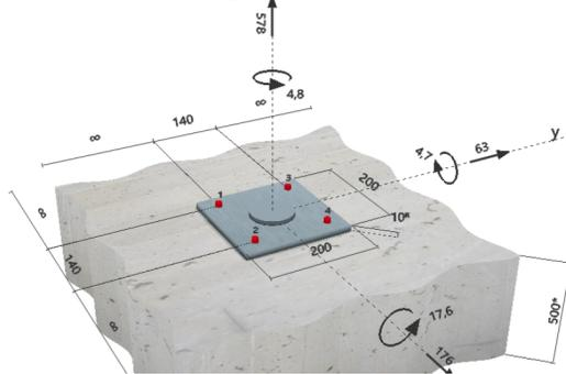
Figure 5: Forces and moment at most loaded feet.
