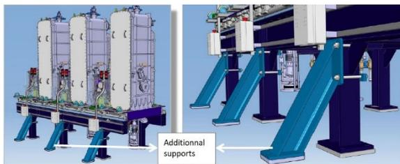
Figure 1: Additional supporting features LINAC A.
