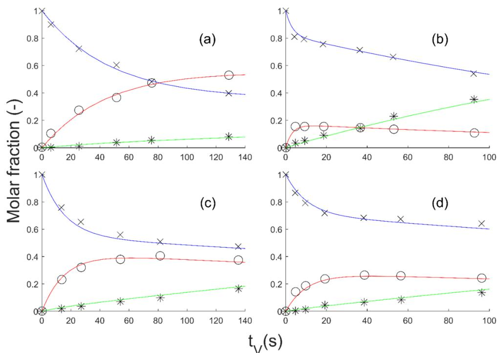
**Figure 4.** Simulation of the extrapolation of Model 3 with the adjusted parameters. GBL (experimental: times cross; model: blue line), BDO (experimental: circle; model: red line) and side products (experimental: star; model: green line) molar fraction vs. time on stream ( $t_V$ ): (a) 35 bar, 200 °C; (b) 25 bar, 240 °C; (c) 35 bar, 220 °C; (d) 25 bar, 220 °C.
