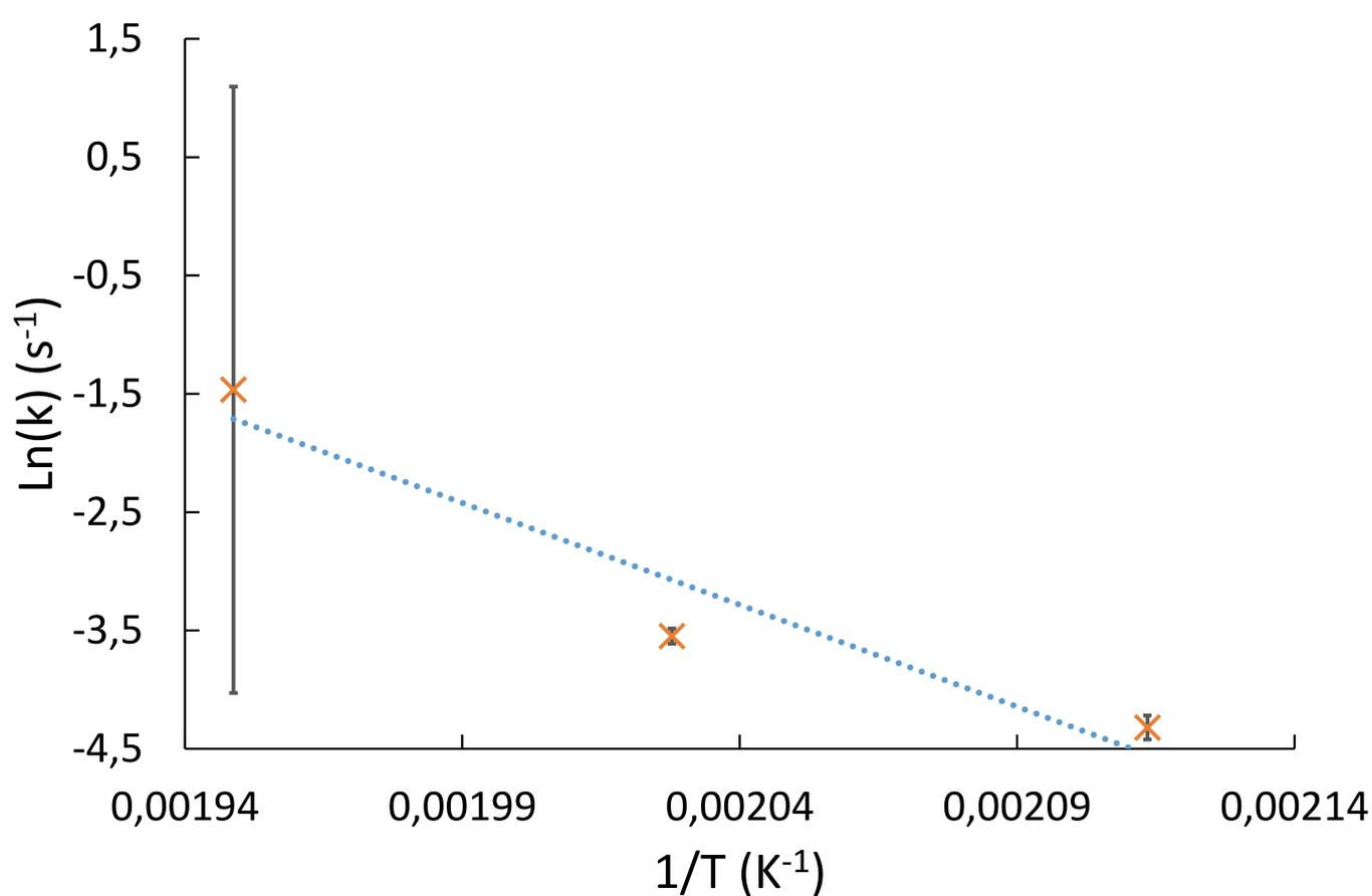
**Figure 3.** Exponential fitting of  $k$  constants of Model 3 between 200 and 240 °C before adjustment.
