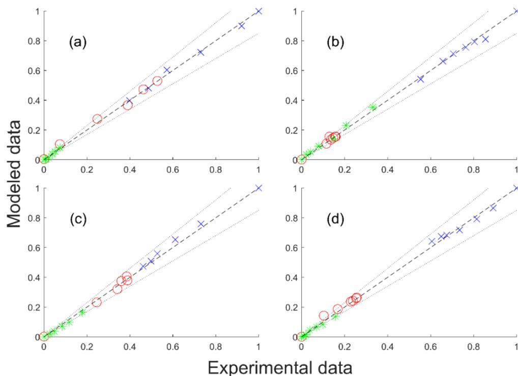
**Figure 5.** Parity diagram of the extrapolation of Model 3 with the adjusted parameters. GBL (blue times cross), BDO (red circle) and side products (green star). Experimental molar fraction vs. modeled molar fraction: (a) 35 bar, 200 °C; (b) 25 bar, 240 °C; (c) 35 bar, 220 °C; (d) 25 bar, 220 °C. Dotted lines represent  $\pm 15\%$  deviations.
