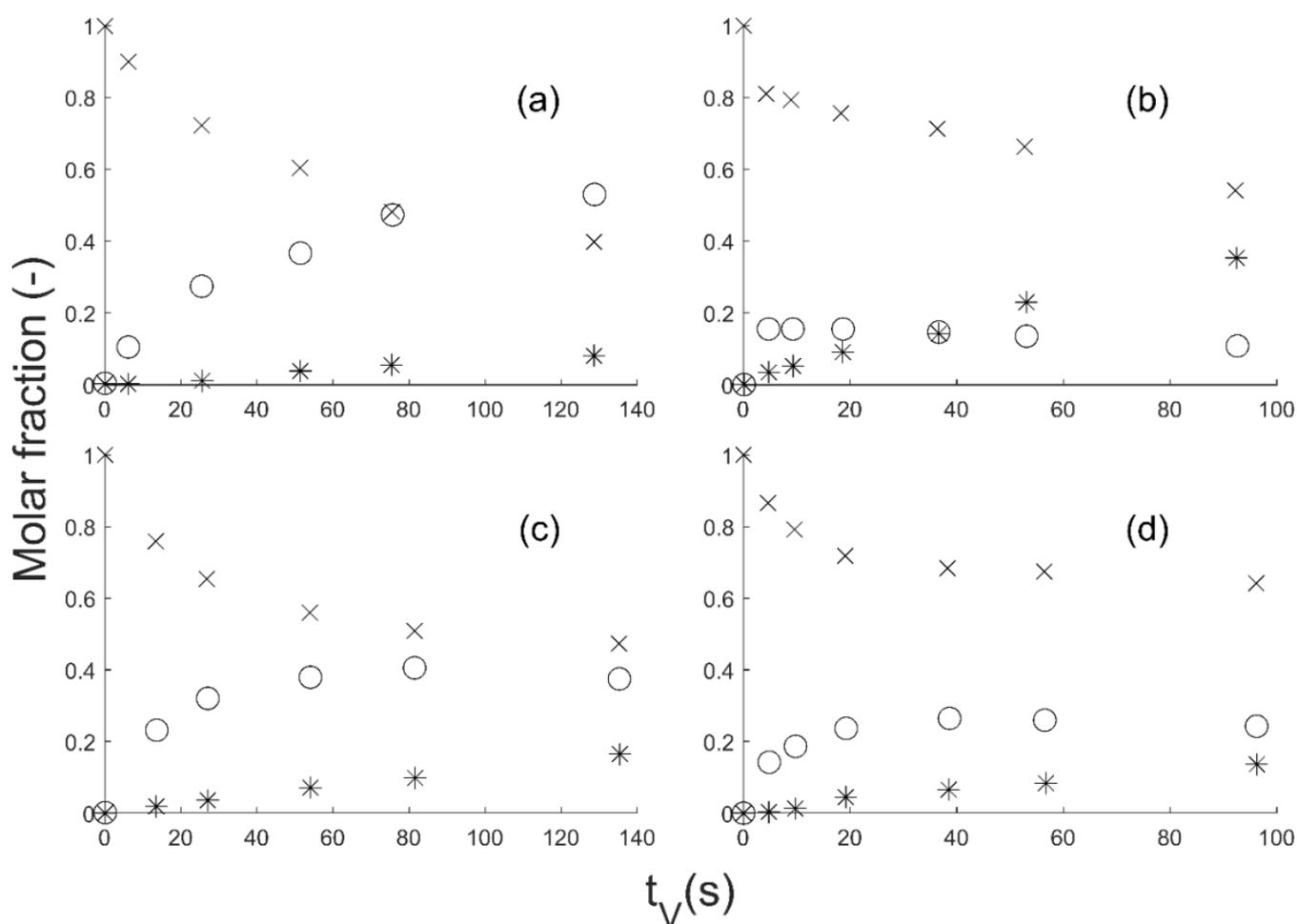
**Figure 2.** GBL (times cross), BDO (circle) and side products (SP) (star) molar fraction vs. time on stream ( $t_V$ ): (a) 35 bar, 200  $^\circ\text{C}$ ; (b) 25 bar, 240  $^\circ\text{C}$ ; (c) 35 bar, 220  $^\circ\text{C}$ ; (d) 25 bar, 220  $^\circ\text{C}$ . The data come from the Ph.D. thesis of J.H. Schlander [25], but were rearranged as a function of  $t_V$  instead of the modified dwell time  $t_{mV}$ .
