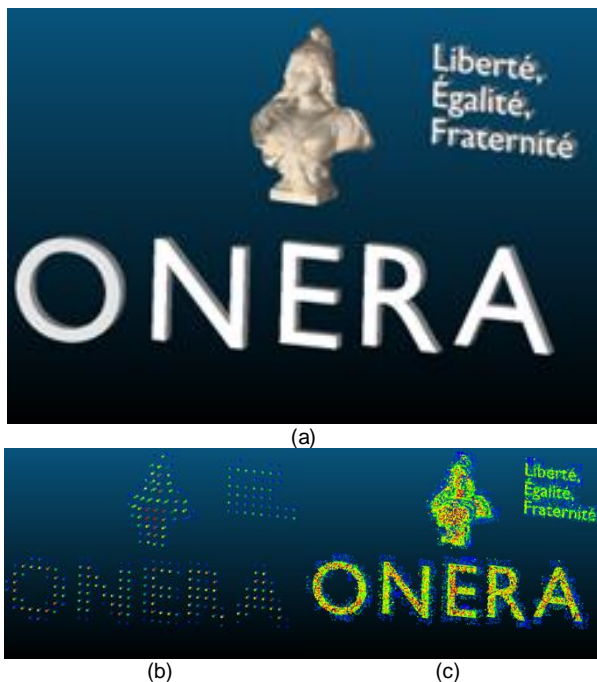
Figure 7 - (a) Original scene, (b) 3D point cloud of a LiDAR (noise removed) and, (c) reconstruction including CS post-processing
