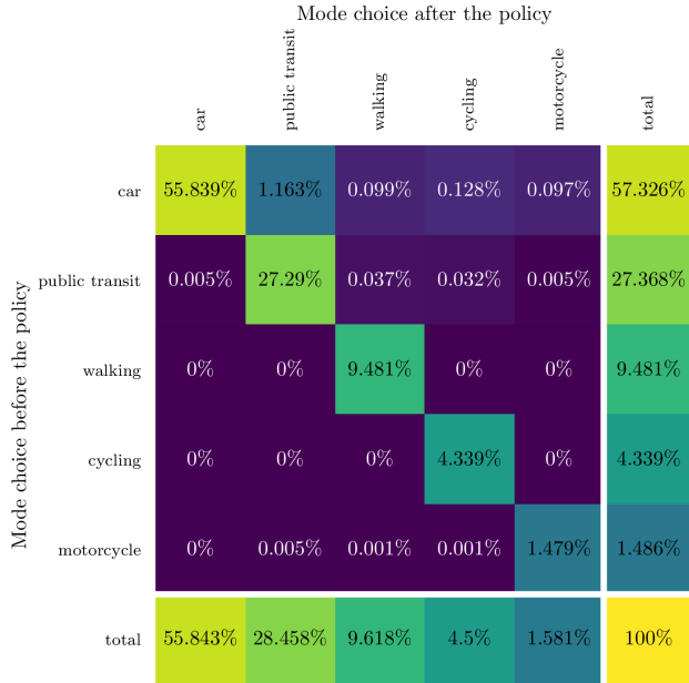
Fig. 5. Evolution of mode share before and after the policy. 1.163% of individuals were given incentives to shift from car to public transit, 27.29% of individuals commuted by public transit before the policy and were not induced to shift.
