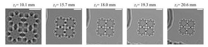
Figure 4 Recorded holograms at different defocusing distances  $(z_1)$  of the 2D test pattern. The white scale bar corresponds to 4  $\mu$ m for all the images.
