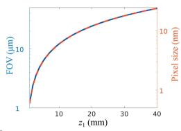
Figure 3 Field of view (FOV) and effective pixel size as a function of the defocusing distance  $(z_1)$  for the NanoMAX in-line holography setup.
