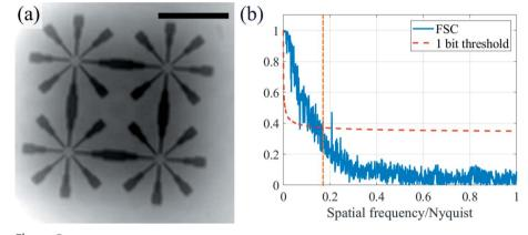
2D test pattern reconstructions (a) and resolution evaluation using Fourier ring correlation (b). The vertical orange-dashed line in (b) represents the focal-spot resolution limit. The scale bar corresponds to 4  $\mu$ m, and the resolution estimated by the 1-bit threshold criterion is 79 nm.
