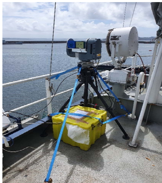
Figure 2: SIMAGAZ instrument (blue one) integrated on a stabilised platform on-board CEPPOL vessel during the experiment.
