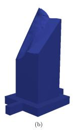
Fig. 22 Fracture surface observed experimentally (Barr and Brokenshire 1996) (a), and obtained by means of the Fast Marching Method (b).
