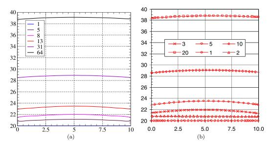
**Fig. 19** Crack front plots, coordinate y as a function of the coordinate z: (a) results obtained using the Fast Marching Method, (b) results obtained by Citarella and Buchhloz (2008). The legend gives the growth increment corresponding to each position of the crack front.
