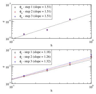
**Fig. 15** Error in terms of  $L^1$  norm for the level set functions as a function of the normalized mesh size, obtained without the treatment of obtuse tetrahedra: normal level set function (top) and tangential level set function (bottom).
