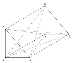
Fig. 11 Spliting of a pentahedron into pyramids.
