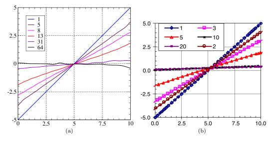
**Fig. 20** Crack front plots, coordinate x as a function of the coordinate z: (a) results obtained using the Fast Marching Method, (b) results obtained by Citarella and Buchhloz (2008). The legend gives the growth increment corresponding to each position of the crack front.
