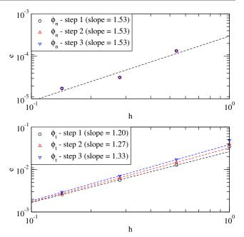
Fig. 14 Error in terms of  $L^1$  norm for the level set functions as a function of the normalized mesh size, obtained with the treatment of obtuse tetrahedra: normal level set function (top) and tangential level set function (bottom).
