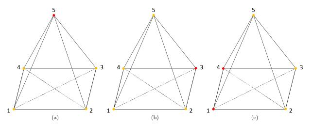
Fig. 10 Spliting a pyramid into tetrahedra. Orange nodes represent known level sets values and red nodes represent level sets values to be determined.
