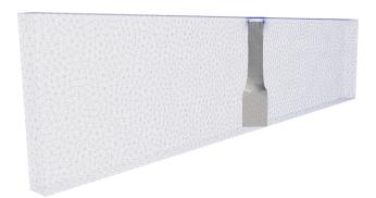
**Fig. 18** Crack path obtained at the end of the simulation of the three-point bending test.
