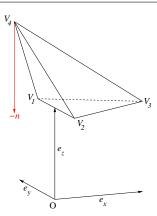
Fig. 8 Illustration of a configuration for which distance  $d_4$  can not be computed using the tridimensional update. The monotonicity condition is not fullfilled, since  $-\mathbf{n} = -\nabla \mathbf{d}(\mathbf{V_4})$  does not lie in convex cone  $\mathcal{C}$ .
