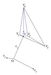
Fig. 9 Illustration of the result of the bidimensional update for face  $V_1V_2V_4$  in the configuration for which the tridimensional update fails. Distance  $d_4$  can be computed because the monotonicity condition is fullfilled, since  $-\mathbf{n}' = -\nabla \mathbf{d}(\mathbf{V_4})$  lies in convex cone  $\mathcal{C}$ .
