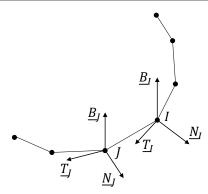
Fig. 1 Discretized crack front and local frame associated with each point on the crack front.
