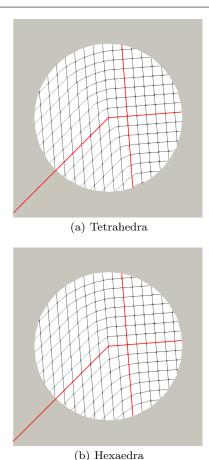
Fig. 13 Representation of the level sets of the normal and tangential level set functions computed at the end of the crack growth using the Fast Marching Method for the update step and applied to: (a) the mesh made of tetrahedra and (b) the mesh made of heaxaedra. The zero level sets of the two level set functions are shown in red.
