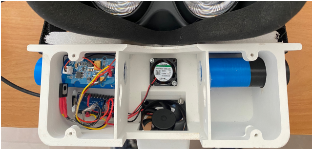
Figure 3: Internal view of our device. Note that we consider only the diffusion of one single odor in this paper (using the left part of the device) ; however, the design allows the diffusion of two odors simultaneously by equipping the right part of the device.
