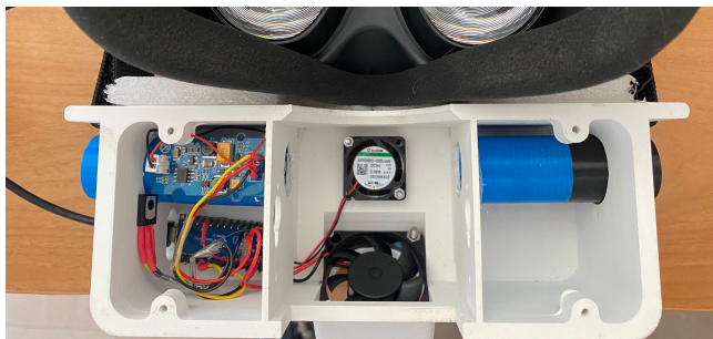
Figure 3: Internal view of our device. Note that we consider only the diffusion of one single odor in this paper (using the left part of the device) ; however, the design allows the diffusion of two odors simultaneously by equipping the right part of the device.
