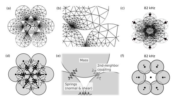
Figure 4: Finite Elements versus Discrete Elements representations of a seven-wire strand. (c) and (f): The normal mode responsible for the "notch frequency" phenomenon for an applied strain of  $\epsilon=0.6\%$ . (d) and (e): In contrast to the intuitive case of contacts between spheres or 3D shapes that are represented with local springs, 2nd neighbors are here directly coupled with non-zero spring constants as a result of line contacts. (a) and (b) adapted from [5].
