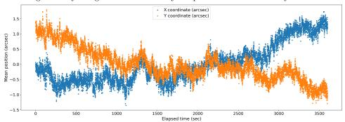
Figure 5. X and Y position measured during one hour on a single target, for testing the tracking accuracy. The values are given in arcseconds on sky.
