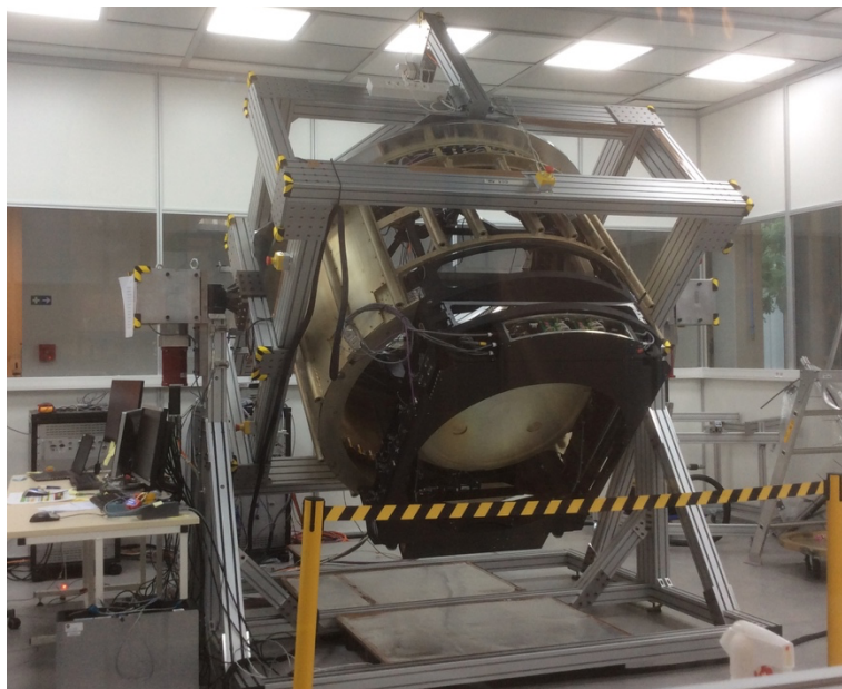
Figure 6. The test-stand holding the full assembly of fake camera body, Carousel and Autochanger, with an angle of -45^\circ on the horizontal axis. The test-stand can rotate along this axis from -90^\circ (pointed vertically, downwards), simulating the camera when the telescope would be pointed at zenith, to +90^\circ , which is not possible for the telescope, but is convenient to perform mechanical work. The whole prototype is additionally mounted over a ring gear, for rotation along the camera axis.
