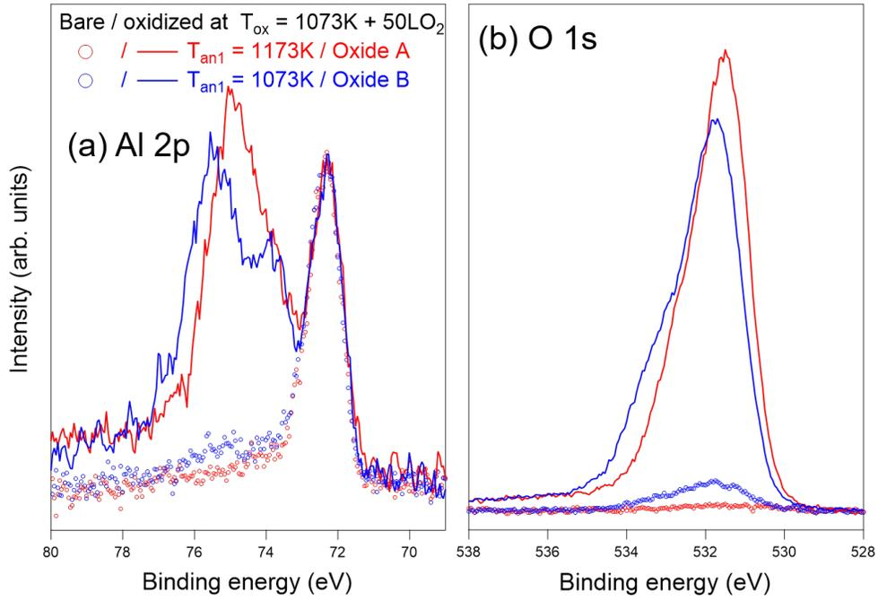
Figure 5: Comparison of XPS core levels of the bare  $Fe_{0.85}Al_{0.15}(110)$  surface to those of the surfaces oxidized at  $T_{ox} = 1073$  K after annealing at either  $T_{an1} = 1193$  K (oxide-A) or  $T_{an1} = 1073$  K (oxide-B): (a) Al 2p; (b) O 1s.
