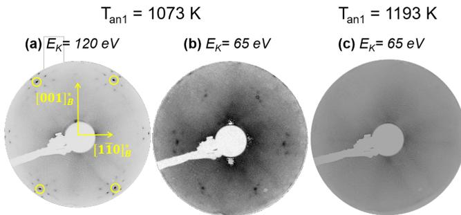
Figure 8: LEED patterns of the  $Fe_{0.85}Al_{0.15}(110)$  surface for beam kinetic energies and annealing temperatures of (a) 120 eV,  $T_{an1} = 1073$  K; (b) 65 eV,  $T_{an1} = 1073$  K; (c) 65 eV,  $T_{an1} = 1193$  K. The active spots of the substrate circled in yellow (Figure a) are surrounded by those of the bare metal reconstruction. Weak spots related to oxide patches show up at 65 eV in (b) for  $T_{an1} = 1073$  K (Figure b) but are absent in (c) after  $T_{an1} = 1193$  K.
