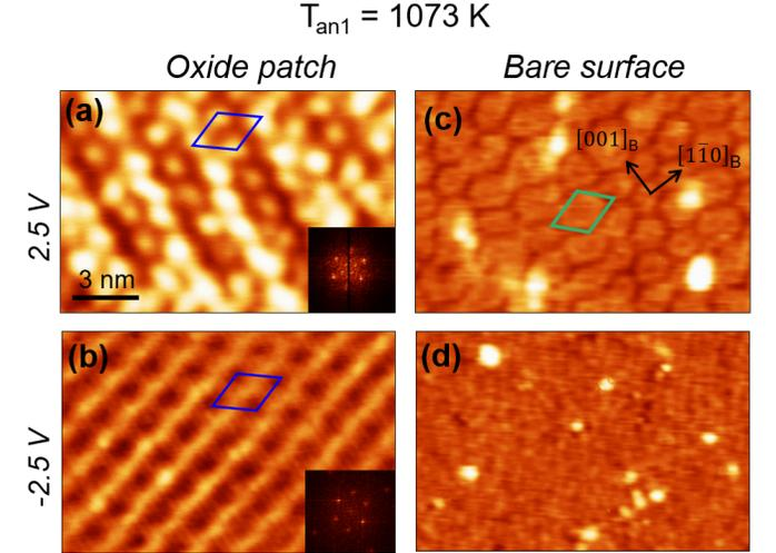
Figure 10:  $(15 \times 15)$   $\text{nm}^2$  STM images of  $\text{Fe}_{0.85}\text{Al}_{0.15}(110)$  surface annealed at  $T_{an1} = 1073$  K: (a)(b) surface structure of patches with Fourier transforms in inset; (c)(d) bare surface. The rhombs evidence the unit cells of the oxide (in blue) and of the bare surface (in green). STM parameters: (a)  $U_b = 2.5$  V,  $I_t = 50$  pA; (b)  $U_b = -2.5$  V,  $I_t = 50$  pA; (c)  $U_b = 2.5$  V,  $I_t = 50$  pA; (d)  $U_b = -2.5$  V,  $I_t = 12$  pA.
