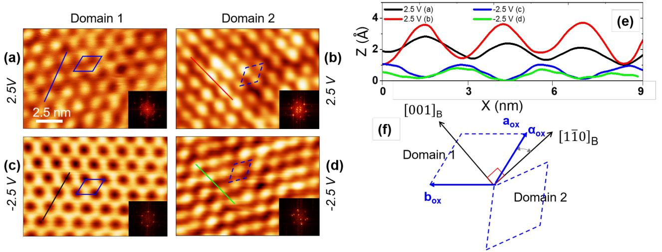
Figure 2: Rotated oxide-B domains shown in Figure 1-d: (a-d) Close-up STM ( $15 \times 10$ )  $\text{nm}^2$  images with Fourier transform in inset (tunnelling parameters : (a)(b)  $U_b = 2.5$  V; (c)(d)  $U_b = -2.5$  V with  $I_t = 50$  pA); (e) Profiles along the lines shown in figures; (f) Scheme of the unit cells of the two oxide domains (blue dotted parallelograms) compared to substrate unit cell (red rectangle).
