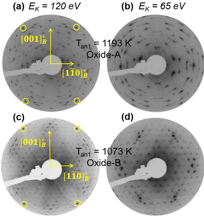
Figure 4: LEED patterns of (a)(b) oxide-A ( $T_{an1} = 1193$  K,  $T_{ox} = 1073$  K) and (c)(d) oxide-B ( $T_{an1} = T_{ox} = 1073$  K) on  $\text{Fe}_{0.85}\text{Al}_{0.15}(110)$  at beam energy (a)(c) 120 eV and (b)(d) 65 eV. Due to the centering of the rectangular surface unit cell of the random  $\text{A}_2$  alloy, only the substrate reflections circled in yellow are visible. Reciprocal surface directions  $[1\bar{1}0]_B^*$  and  $[001]_B^*$  are shown with arrows.
