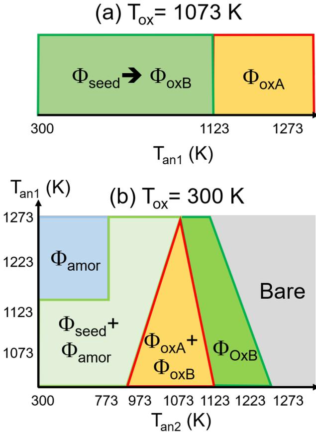
Figure 12: Schematic stability diagram summarizing observations for  $\text{Fe}_{0.85}\text{Al}_{0.15}(110)$  oxidation at (a)  $T_{ox} = 1073$  K and (b)  $T_{ox} = 300$  K after a substrate annealing at  $T_{an1}$  prior to oxidation or after a post-oxidation annealing at  $T_{an2}$ : (i)  $\Phi_{OxA}/\Phi_{OxB}$  correspond to the fully covering oxides, (ii)  $\Phi_{seed}$  to a reconstructed metallic surface covered by B-type oxide patches, (ii)  $\Phi_{amor}$  to the amorphous oxide.
