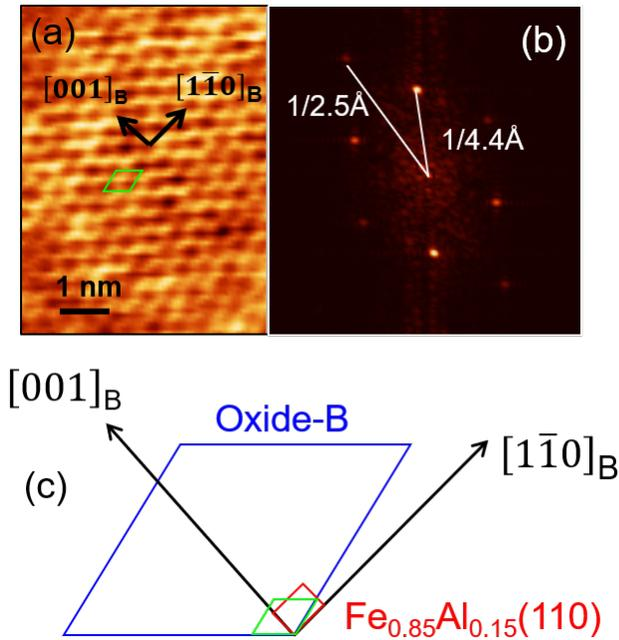
Figure 3: Unit cell of oxide-B: (a) STM at atomic resolution of the alumina film ( $U_b = 0.5$  V,  $I_t = 12$  pA); (b) Fourier transform that shows a  $\sim 4.4$  Å hexagonal periodicity; (c) oxide, substrate, atomic network unit cells represented by blue, red and green parallelograms, respectively.
