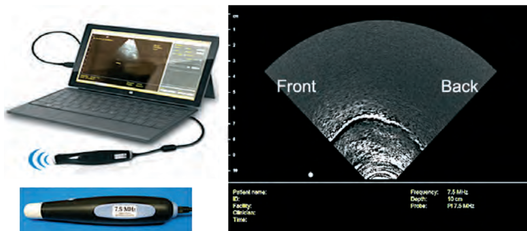
Fig. 1: SeeMore probe ( https://seemore.ca/portable-ultrasound-products/pi-7-5-mhz-speech-language-pathology-99-5544-can/ ) with illustration of portable ultrasound system (left), and display of tongue contour (sagittal plane) during the production of /æ/ in “cat” by speaker FR3 (right) (photo by Barbara Kühnert and Claire Pillot-Loiseau).
