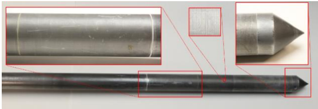
Fig. 3. Simplified cross-section and view of the instrumented pile-probe
