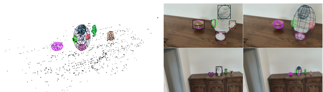
Figure 12: Illustration of by-part modeling. Left: reconstructed map. Right: localized images using complete objects (bottom row) or parts (top row).
