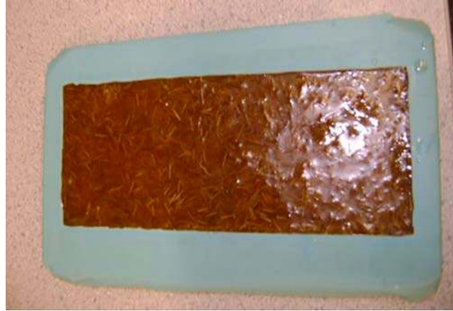
Fig. 3. Alfa/Epoxy composite mold.
