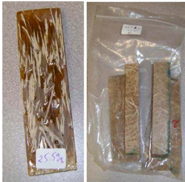
Fig. 4. Alfa/Epoxy test specimen's.
