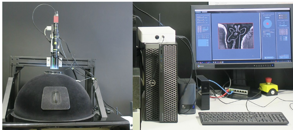
Fig. 1 The RTI dome used for data acquisition (at ImViA Laboratory, France)
