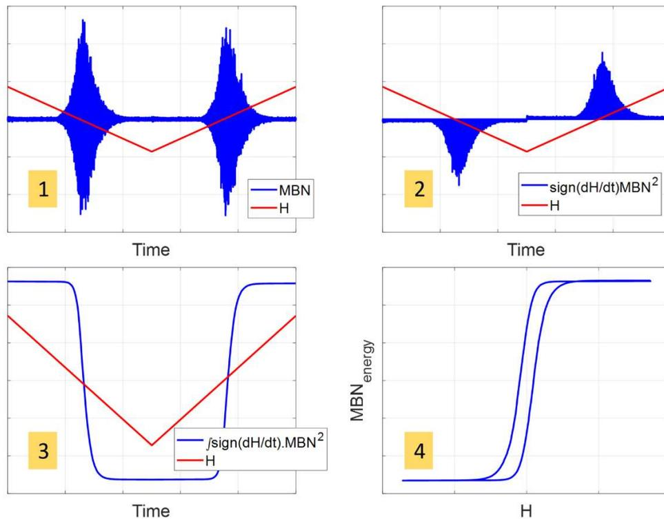
Fig. 4 –  $MBN_{energy}(H)$  hysteresis loop, construction process.
