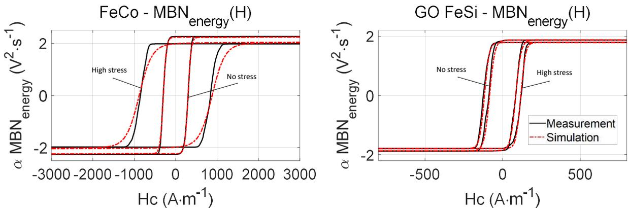
Fig. 10 Comparisons simulations/measurements for the  $MBN_{energy}(H)$  hysteresis cycles.
