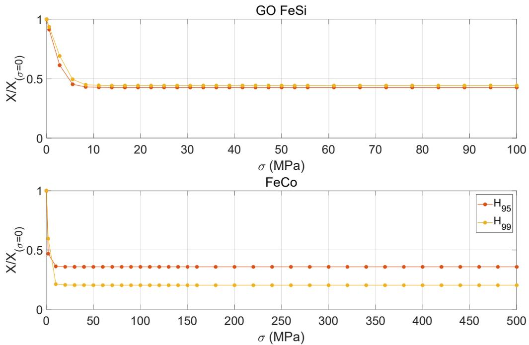
Fig. 12 – Multiscale model prediction  $H_{95}$  and  $H_{99}$  normalized by the corresponding stress-free reference, as a function of the applied tensile stress.
