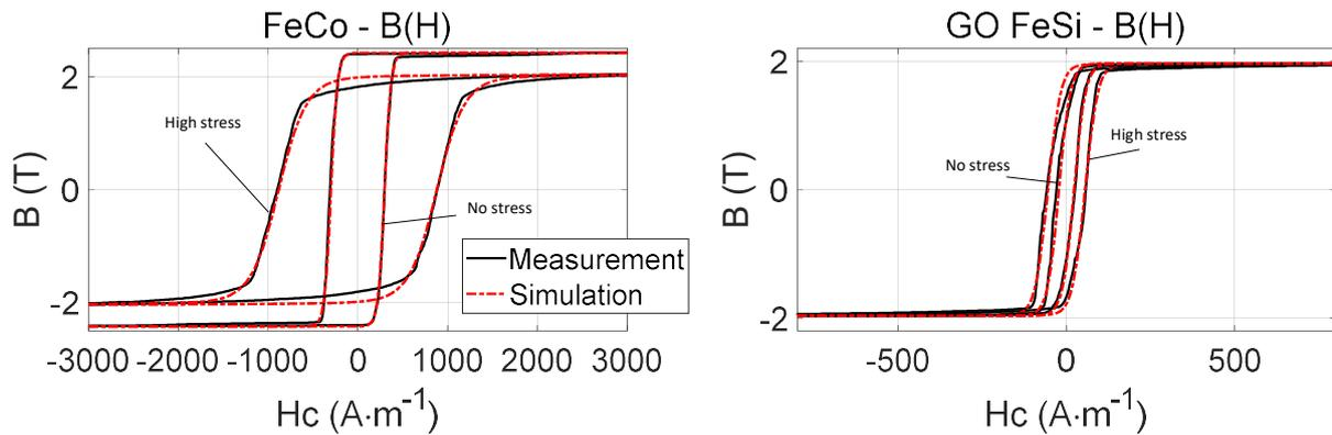
Fig. 9 Comparisons simulations/measurements for the  $B(H)$  hysteresis cycles.
