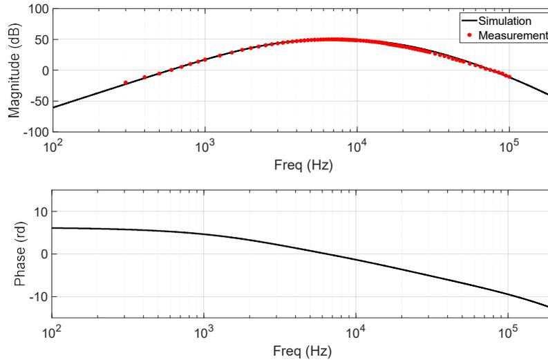
Fig. 8 – MAX274ACN analogic filter Bode plots, comparison measurement/simulation.
