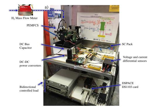
Fig. 8. Laboratory experimental setup of the FC/SC hybrid system
