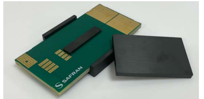
Fig. 1: A planar high frequency power transformer.
