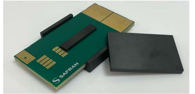
Fig. 1: A planar high frequency power transformer.
