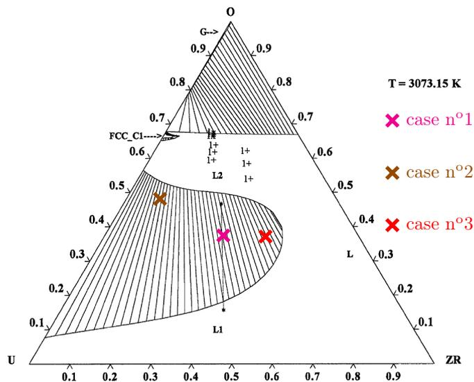
Figure 1: U-O-Zr phase diagram at temperature  $T = 3073.15\text{K}$  and pressure of 1 bar (adapted from [17]) and locations associated with the system inventory for the different simulations of Section 3.
