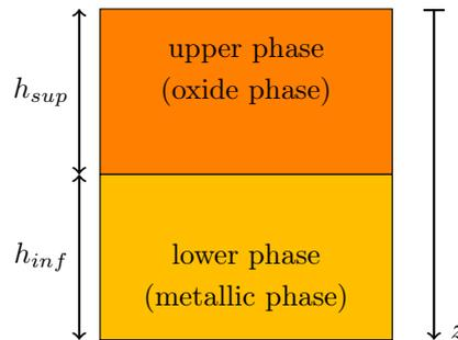
Figure 3: Schematics of the 1D simulation setup
