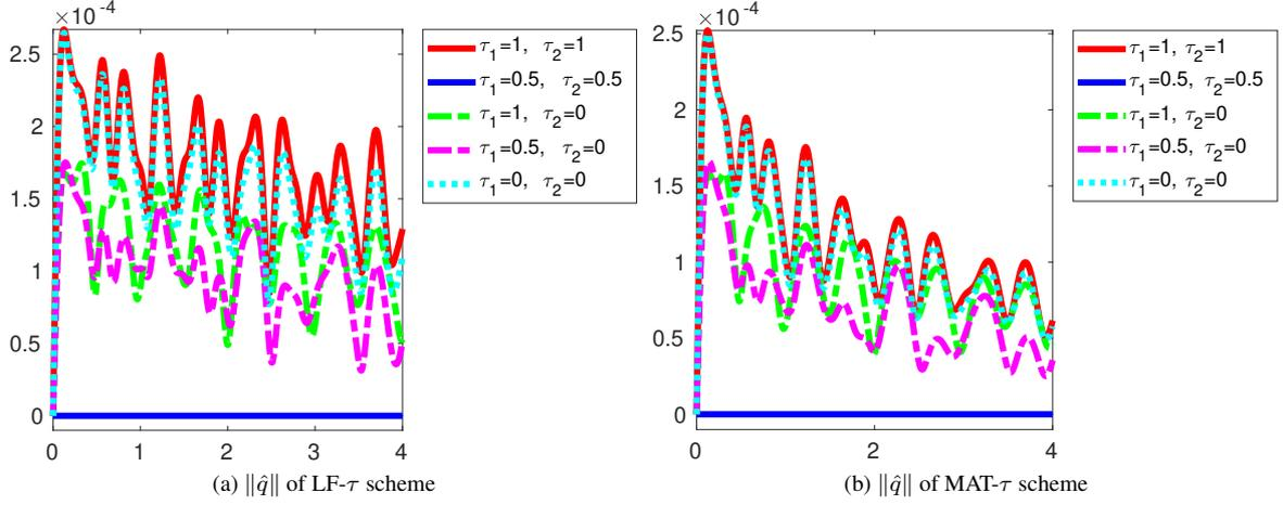
Figure 6: Orthogonality preserving test case: evolution of the kernel part of the LF- $\theta$ - $\tau$  and MAT- $\theta$ - $\tau$  scheme with  $\theta_1 = \theta_2 = \frac{1}{2}$  and various values of  $(\tau_1, \tau_2)$ . Orthogonality preservation is only achieved when  $\tau = \theta$ .
