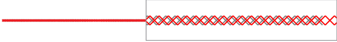
Fig. 4. Extensional mode (mode 10 in Fig. 3) for the considered p-beam. Red and gray colors denote the natural modes and the initial configuration, respectively. (For interpretation of the references to color in this figure legend, the reader is referred to the web version of this article.)
