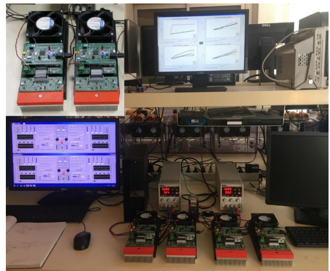
Figure 18. Test platform for ageing of samples
