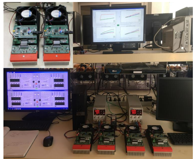
Figure 18. Test platform for ageing of samples
