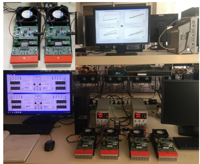
Figure 18. Test platform for ageing of samples
