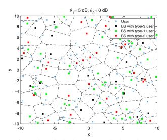
**Fig. 1** PPP deployment for BS with a randomly selected user in each cell. Fig. 1 illustrates one realization of a PPP network for three types of served users, with only one user per BS represented by *X*. The BS colored in green, red and black represent the active BS for users of type 1, type 2 and type 3, respectively.
