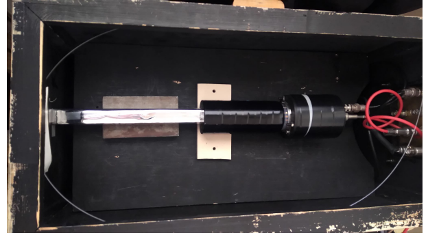
Figure 4: Setup of the light yield test. The crystal wrapped with VM2000 and attached to a PMT. Everything is placed in a dark box. The radioactive source was attached to the end of the crystal.
