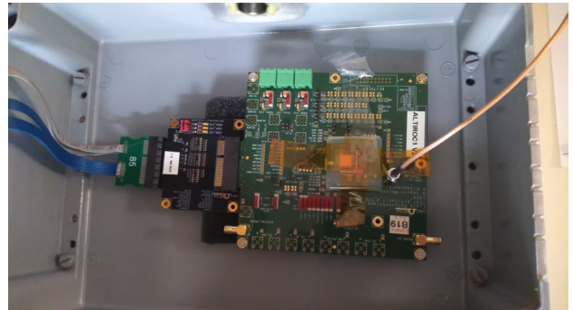
Figure 9: Test board with an AC-LGAD sensor and the ALTIROC readout chip placed inside the dark box.
