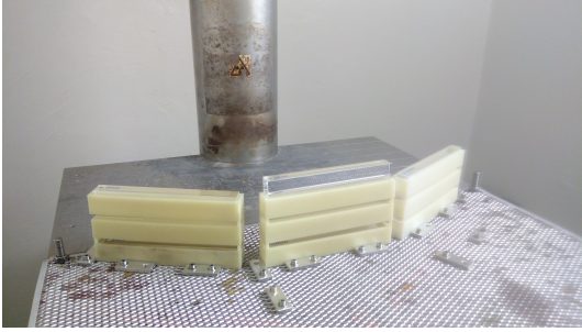
Figure 2: Experimental setup for radiation hardness measurements. The crystals are placed in front of a strong ^{60}\text{Co} source, which is inside the vertical cylinder. Different radiation dose rates can be achieved by changing the distance between crystals and the ^{60}\text{Co} source.
