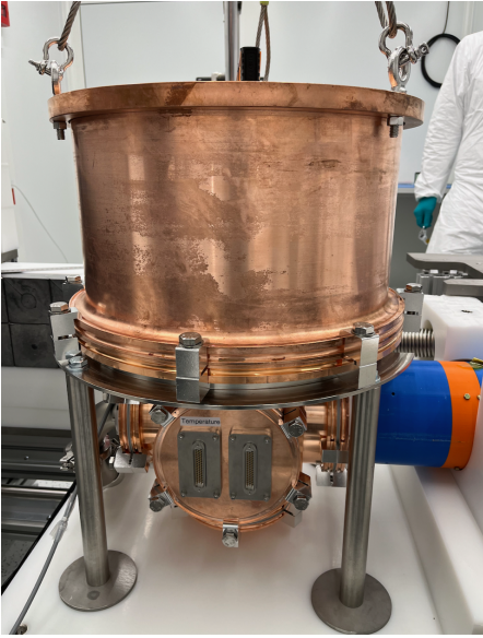
Figure 2: The Low Background Chamber prototype installed at the LSM.
