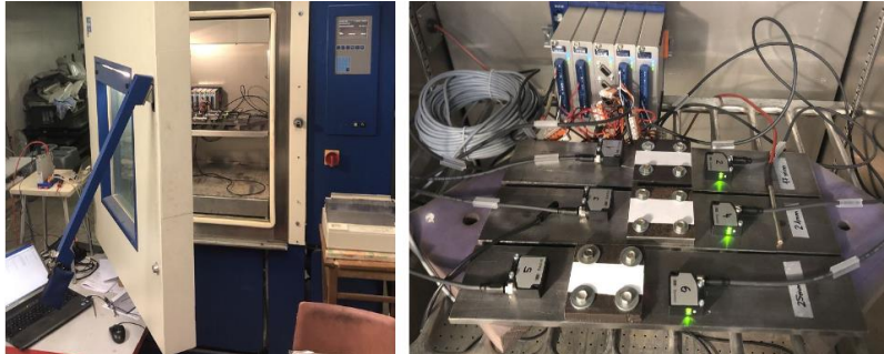
Figure 1: Experimental setup for Laser Triangulation Sensors within the climate chamber
