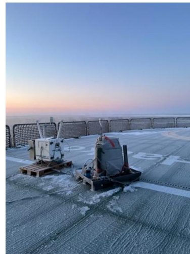
Figure 1- Path of cruise during the campaign (left), the dotted lines indicate the periods when systems were not operating. Lidars positioning and setup on board R/V Kronprins Haakon (right).
