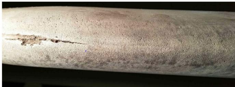
Figure 1: Eroded leading edge (by Christian Bak) [1]
