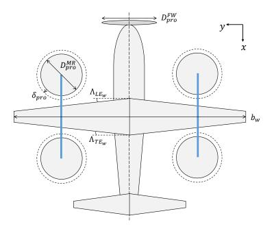
Figure 2 – VTOL propellers location for FW-VTOL geometry
