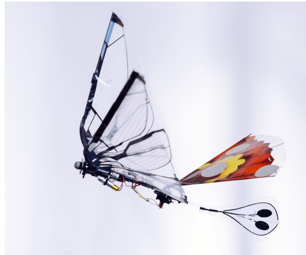
Fig. 1. The 10-gram Metafly Flapping-Wing Micro Aerial Vehicle in the Marseille flight arena © Cyril Frésillon / ISM / CNRS Photothèque
