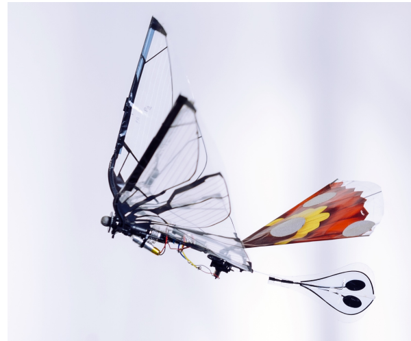
Fig. 1. The 10-gram Metafly Flapping-Wings Aerial Vehicle in Marseille's flight arena © Cyril Frésillon / ISM / CNRS Photothèque
