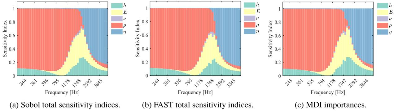
Figure 3: Total sensitivity indexes of the STL analyses for isotropic plates.
