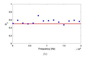
Figure 14: Identified values of  $a_0$  (a) and  $D_y$  (b) calculated using the identification method on the solution fields at different frequencies, exact values (-) and identified values ( $\bullet$ )
