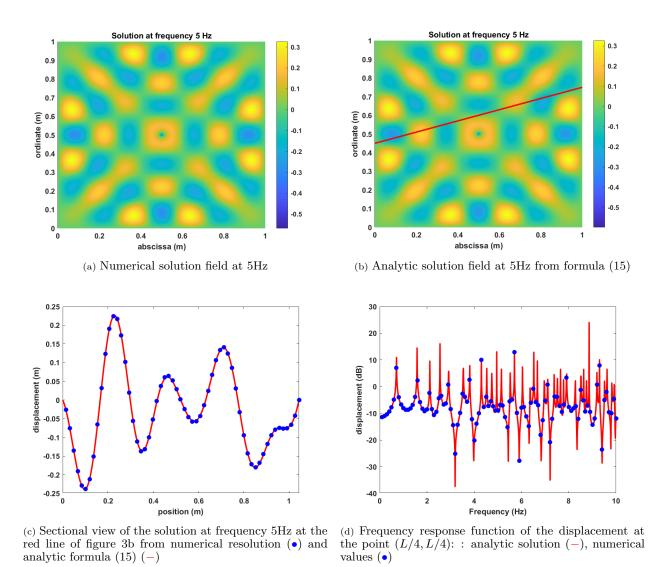
Figure 3: Comparison between analytic and numerical solutions: solution fields at 5 Hz, (a) numeric, (b) analytic, (c) displacement function of the position, (d) frequency response function
