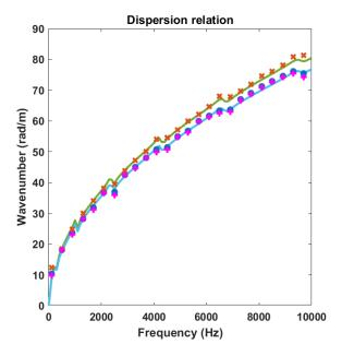
Figure 16: Dispersion relation, analytic and from INCOME of the equation (33) in the directions 0,  $\frac{\pi}{4}$  and  $\frac{\pi}{2}$ : analytic dispersion relation at 0 rad (-),  $\frac{\pi}{4}$  rad (-),  $\frac{\pi}{2}$  rad (-), INCOME wavenumbers at 0 rad (•),  $\frac{\pi}{4}$  rad (×) and  $\frac{\pi}{2}$  rad (+)
