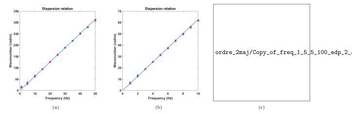
Figure 6: Dispersion relation, analytic and from INCOME for the  $2^{nd}$ -order equation with  $a_x=1$ ,  $a_y=1$ ,  $a_{xy}=0$  and  $a_0=1$ : analytic dispersion relation (–), INCOME wavenumbers at angles 0 rad (•),  $\frac{\pi}{4}$  rad (×) and  $\frac{\pi}{2}$  rad (+). (a): L=1m on a grid of 400 by 400 points, (b): L=5m on a grid of 400 by 400 points and (c): L=1m on a grid of 60 by 60 points.
