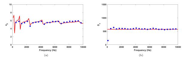
Figure 17: Identified values of  $a_0$  (a) and  $D_x$  (b) calculated using the identification method on the solution fields for frequencies below 10 kHz, exact values ( $\bullet$ ) and identified values ( $\bullet$ )
