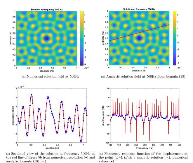
Figure 5: Comparison between analytic and numerical solutions: solution fields at 500 Hz, (a) numeric, (b) analytic, (c) displacement function of the position, (d) frequency response function
