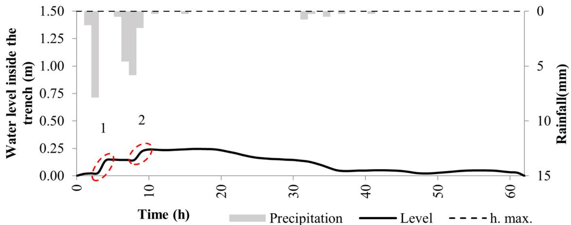
Figure 7. Infiltration trench event 2 (E2) from 29 April to 2 May from 2017. The different numbers correspond to the different parts of the curves that are discussed in the text.
