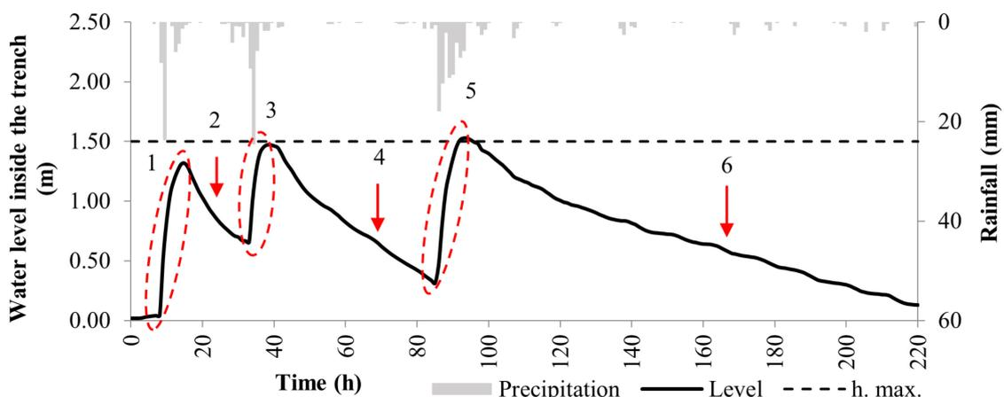
**Figure 9.** Infiltration trench event 4 (E4) from 27 May to 5 June 2017. The different numbers correspond to the different parts of the curves that are discussed in the text.
